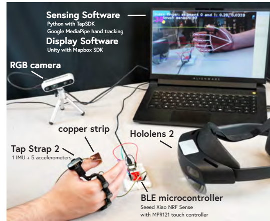
Figure 6: The gesture set (left) and hardware setup (right) for our proof-of-concept prototype.
