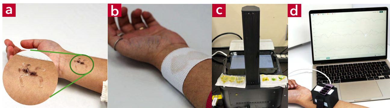
Figure 1: We contribute sustainable fabrication of biochemical holographic sensors derived from bacteria, enzymes and organic biochemical sources. These open up new avenues for biological and environmental sensing for HCI. (a) A biochemical sensor made from flavin enzyme derived from Aerococcus viridans bacteria. It measures the lactate levels in the sweat to indicate the intensity of physical activities. (b) A wearable sweat sensor that is functionalized with a glucose-sensing assay derived from Aspergillus niger mold. (c) We also demonstrate the fabrication of gas sensors. Carbon dioxide sensors made on diverse soft biodegradable, bio-sourced and vegan-friendly material substrates visually indicating the amounts of carbon dioxide emissions from an SLA printer (darker the yellow tone, higher the emissions). (d) Low-cost, wearable holographic sensing for self-contained real-time quantitative data streaming.
